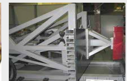
Intrusion tests 200kN
